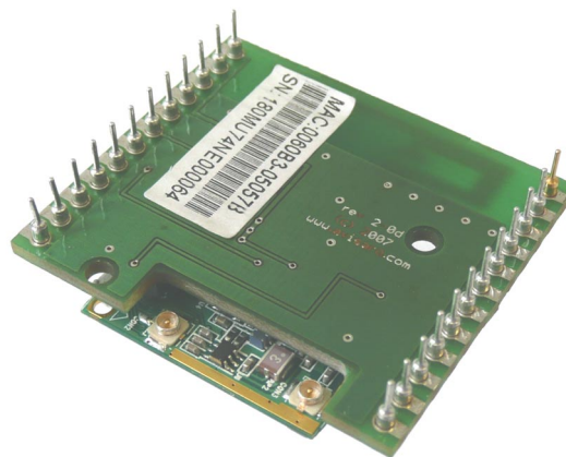
The reverse side with the U.FL antenna connectors
